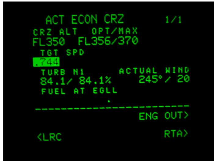
Fig. 17.2.4.2 Boeing 737 Flight Management Computer: Cruise Display (This photo was taken before 2005)
